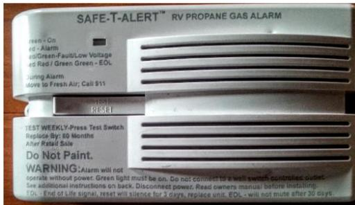
Each RV is equipped with a propane detector, located near the floor. The alarm goes off whenever an increased propane emission (e.g., from the stove or oven) is detected. Please make sure not to place any objects on the propane detector to avoid false alarms.
