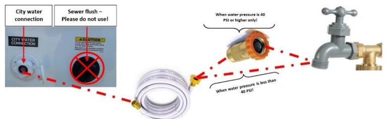
3. Connect the other end of your water hose to the water pressure regulator and the regulator to the water tap of the camp site when the water pressure is 40 PSI or higher. If the pressure is lower than 40 PSI, connect the other end of the hose directly to the tap.
