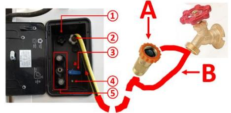
To **FILL THE FRESHWATER TANK**, follow steps 1 to 3 above. Then put the selector lever ③ to position **a**!
