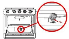
The pilot light is underneath the tray in the back of the oven. To light the oven, turn the oven knob to the PILOT ON position and keep it pressed in. At the same time, light the pilot light using a gas lighter. Wait for about 1 minute, then slowly release the knob while turning it to the desired oven temperature. The burner will now fully ignite. Turn the knob back into the OFF position to turn off the oven.
