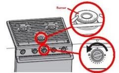
Press in the knob of the corresponding element and turn it counter-clockwise (propane flow can be heard). Ignite the element by turning the spark knob or using a gas lighter. Turn the element's knob to desired level and release. To shut off an element, turn the corresponding knob back to the OFF position. Be sure that the knob clicks into place and is locked so it can no longer be turned.
