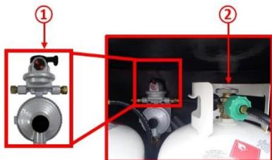
Stove top burners, oven, water heater, furnace and refrigerator are operational by propane operated. To ensure that sufficient propane is available, the camper is equipped with two propane bottles which are located in one of the external compartments of the camper. The main valve ① for the propane supply is directly on the tank. The small black lever ② must point to the open bottle. Otherwise, the gas flow is blocked.
