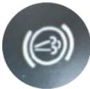
The diesel engine brake can be used together with the Tow/Haul function. When activated, braking assistance from the engine is boosted providing enhanced handling and control, and reduced brake and transmission wear while going downhill. Press the button on the dashboard to switch the function ON or OFF.
